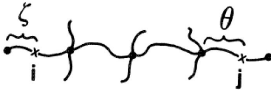
Fig 6. Two points i and j of the network separated by d = 3 tetrafunctional junctions. The positions of points i and j are measured with respect to the nearest multifunctional junction from the left as fractions \zeta \theta of the contour length of the chain between multifunctional junctions.
