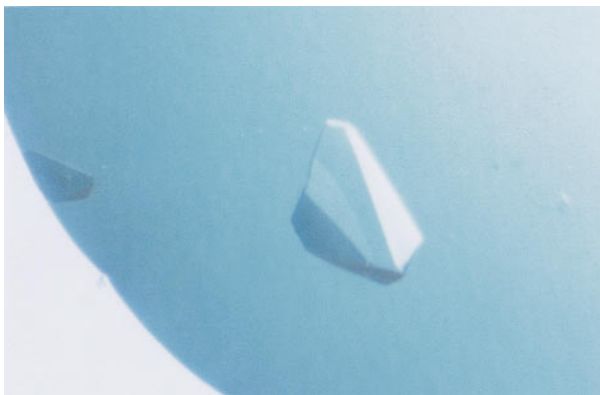
FIG. 6. Crystal of Src- \Delta U phosphorylated at Tyr-527. The crystal was grown in a hanging drop and grew in 3 days at 4°C. The drop contained 100 mM Tris-HCl, 20% PEG2000, 5% 2-methyl-2,4-pentenediol, 200 mM NaCl, 5 mM DTT, 1 mM sodium azide, and 0.1 mM sodium orthovanadate. In the longest dimension the crystal measures 0.4 mm.
