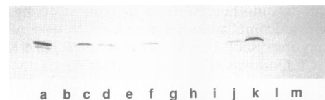
FIG. 3. Western blot analysis of cell envelope fractions with anti-PldA serum. Applied was 0.01 µg of purified E. coli PldA protein (a) or cell envelope fractions of K. pneumoniae (b), C. freundii (c), Shigella flexneri (d), Erwinia herbicola (e), Serratia marcescens (f), Providencia stuartii (g), Edwardsiella tarda (h), Yersinia enterocolitica (i), Enterobacter aerogenes (j), S. typhimurium (k), P. vulgaris (l), or Enterobacter cloacae (m).
