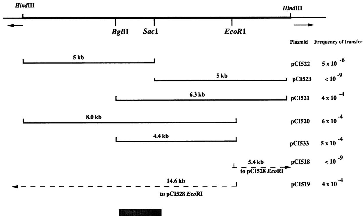
FIG. 3. Restriction map of 10-kb *Hind*III fragment of pCI528. —, pCI528 DNA; —, pCI3340/pCI372 DNA. Solid line segments, subfragments of the 10-kb fragment of pCI528 cloned into pCI3340/pCI372; broken line segments, flanking *Eco*RI fragments cloned into pAM401; ■, consensus transfer region. Transfer frequencies of subclones are listed.
