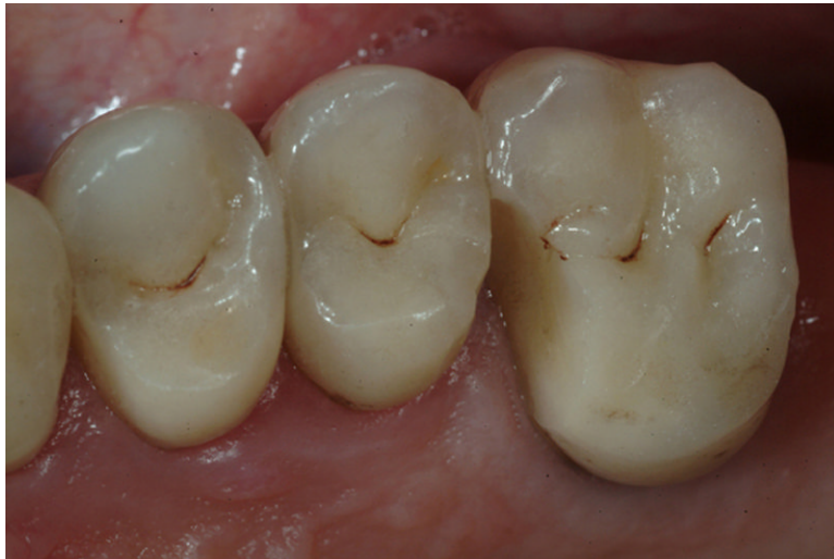
Fig. 1. Fracture of the veneering porcelain (AllCeram) of an upper left Procera alumina molar after 4.2 years of intra-oral function
