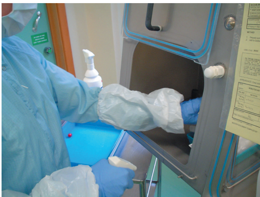
Figure 3 Prepared product being removed from isolator about to be sprayed with alcohol.
