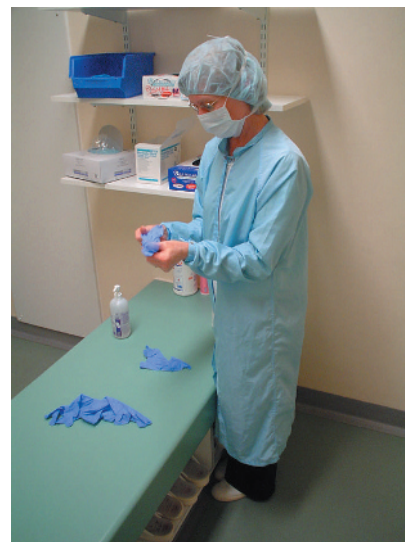
Figure 1 Clean-room worker gowning and gloving on the "clean-room" side of the changing room.
