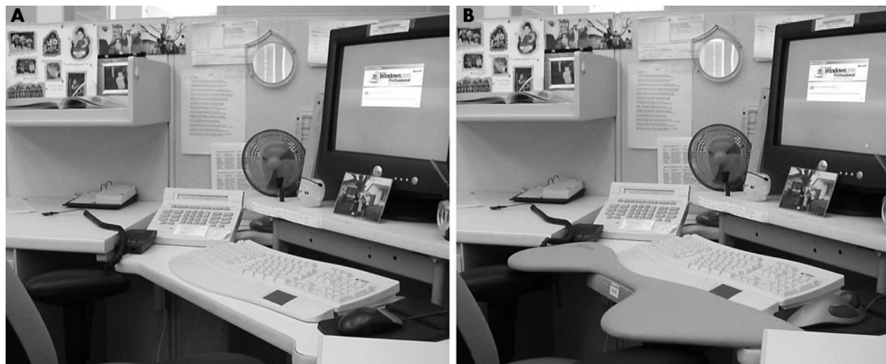
Figure 1 Examples of two of the workstation interventions: (A) no equipment changes; (B) forearm support board and trackball.
