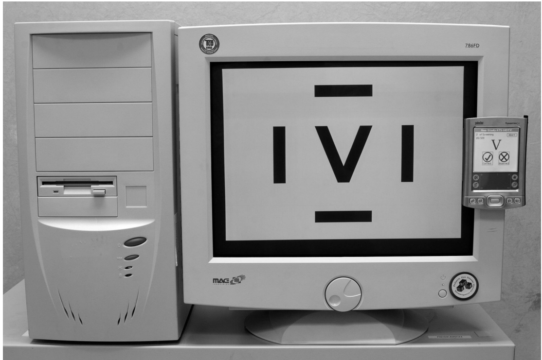
Figure 1. Amblyopia Treatment Study HOTV Visual Acuity Testing Protocol Presented on the Electronic Visual Acuity (EVA) Tester
