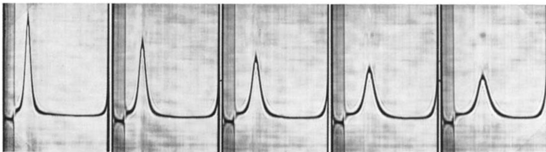
FIGURE 18 Analytical centrifugation pattern of purified glycogen particles. A 1% glycogen aqueous solution was centrifuged in a Spinco model E ultracentrifuge at 17,980 rpm. Photographs were taken at 4-min intervals.
