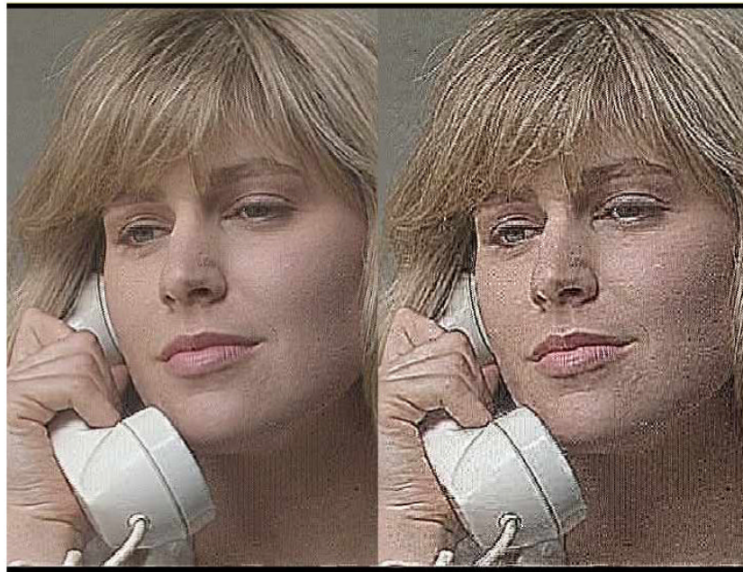
Fig. 4. Illustration of the side-by-side video segments used to determine the just noticeable differences (JNDs) in levels of MPEG-enhancement in the third preliminary experiment. In this example the reference video is on the left, with k = 11.8 . The level of enhancement of the stimulus video on the right alternated every 850ms between that of the reference video and a test level. The test level of enhancement was increased or decreased at every flicker cycle until the observer correctly reported the side that was flickering. The difference between the reference and test k at that time was the JND. The image shown on the right ( k = 35.4 ) represents 4 JNDs, as a single JND is hard to appreciate in the print.
