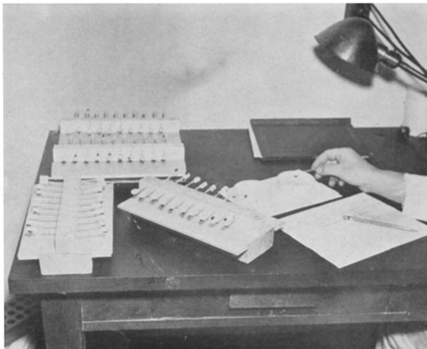
FIG. 5. Experimental arrangement, showing fly racks, a fly being fed, and record sheet.
