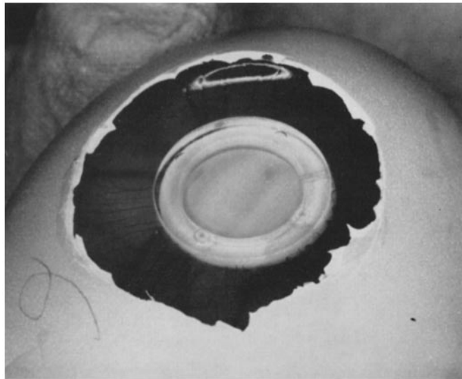
FIG. 1. Diffusion chamber embedded in chorioallantois. The circular cover slip sealing the hole in the shell has been removed and the hole enlarged to expose the chamber.
