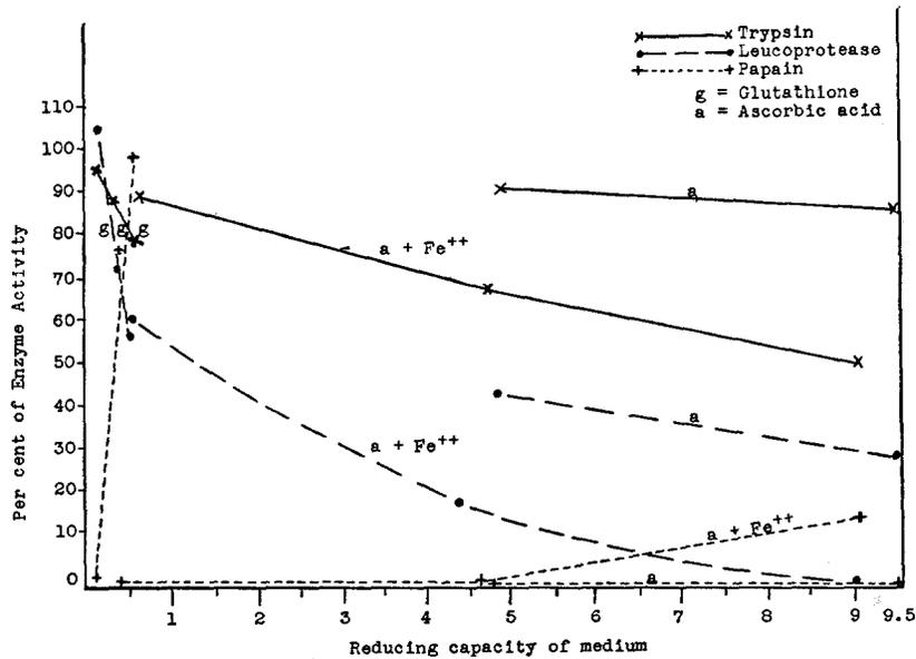
CHART 2. The influence of reducing agents (glutathione, ascorbic acid, and ascorbic acid + Fe<sup>++</sup>) on the activity of leucoprotease, crude trypsin, and papain. (The reducing capacity of the medium is recorded as the cubic centimeters of 0.0005 M Na-2,6-dichlorophenol indophenol decolorized by 1 cc. of digest mixture.)
