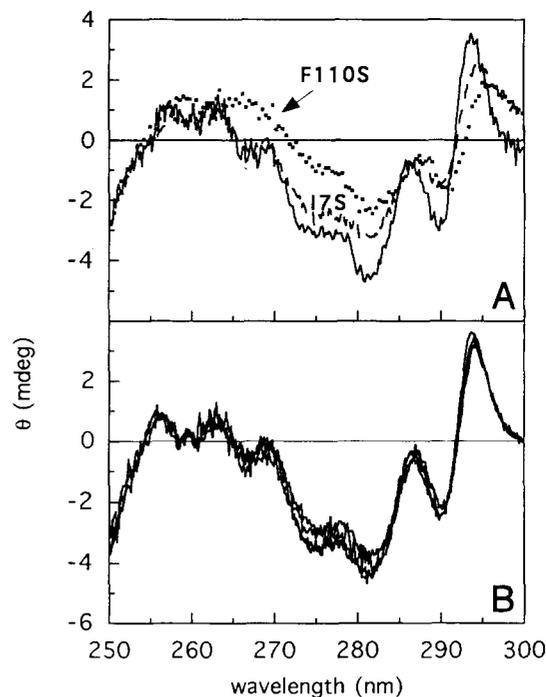
**Fig. 5.** Near-UV CD spectra of (A) apo wt (solid line), I7S (dashed line), F110S (dotted line) samples and (B) apo H35F, H35L, H35Q, and M44K.
