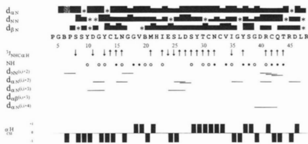
Fig. 4. Summary of NMR data for [Abu6, 20] mEGF4-48 in 90% H 2 O/10% 2 H 2 O at pH 2.8 and 300 K. The intensities of d_{\alpha\text{N}} , d_{\text{NN}} , and d_{\beta\text{N}} connectivities are represented as strong, medium, or weak by the height of the bars. The shaded bar indicates a d_{\alpha\beta} connectivity to Pro7. Asterisks indicate that the presence of a NOE could not be confirmed unambiguously due to peak overlap. Values of ^3J_{\text{NHC}\alpha\text{H}} < 6 Hz are indicated by ↓, those > 8 Hz by ↑. Those left blank could not be measured due to overlap, or were between 6 and 8 Hz. The relative exchange rates of backbone NH protons are indicated in the row labeled NH, based on the strength of cross-peaks in a 2 H 2 O exchange TOCSY experiment; slowly exchanging amides are indicated by filled circles, while open circles indicate intermediate exchange. NH protons with intermediate exchange rates were identified as those that had peaks present in the TOCSY spectra after 10 h but not after 24 h. The bottom plot is a chemical shift index (CSI) analysis (Wishart et al., 1992) for the C ^{\alpha} H resonances, where CSI is shown as positive if the C ^{\alpha} H resonance is > 0.1 ppm downfield from its random coil value (Wishart et al., 1995a), negative if > 0.1 ppm upfield, or 0 if within 0.1 ppm of its random coil value.
