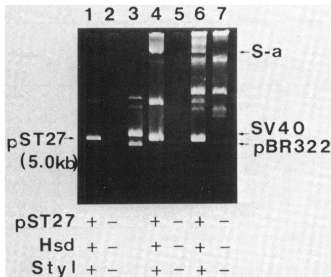
FIG. 2. Occurrence of the 5.0-kb Hsd plasmid (pST27) in StyI endonuclease-producing cells. Plasmid DNA was isolated from the strains by the alkaline lysis method of Maniatis et al. (20). Agarose (1%) gel electrophoresis of the DNAs was carried out at 80 V for 150 min. Lane 1, Salmonella typhi 27; lane 2, Salmonella typhi 27Hsd - ; lane 3, simian virus 40 (SV40) 5.2-kb and pBR322 4.4-kb size standards; lane 4, E. coli WA921 (pST27, S-a); lane 5, E. coli WA921; lane 6, E. coli YY201(pST27, S-a); lane 7, E. coli YY201. The occurrence of host specificity for DNA (Hsd) in these strains was tested by the method of Wood (32), using phage \lambda .0 for E. coli strains and phage ViII.0 for Salmonella typhi strains. We noted that all of the strains carrying the 5.0-kb plasmid had Hsd + characteristics and produced endonuclease StyI ( StyI + ). Although no clear bands were observed in lanes 2 and 5, these cells certainly lysed, since a faint band of chromosomal DNA migrating slightly faster than the plasmid S-a band was observed.
