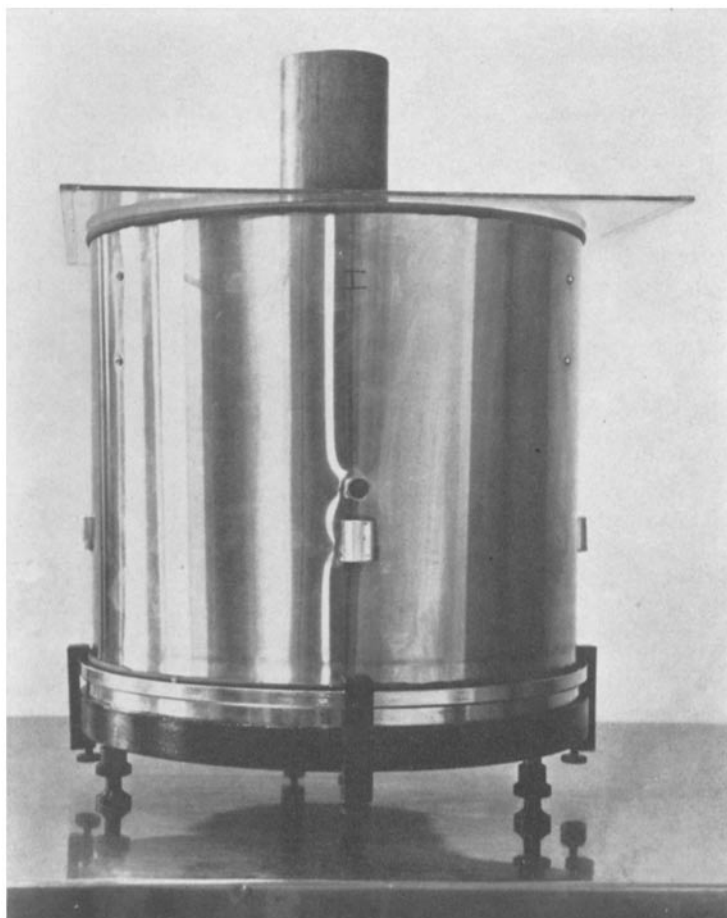
FIG. 2. Elevation view of equipment for collodion membrane casting.
