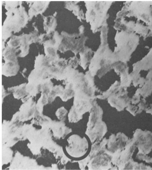
FIG. 7. Oblique section of a collodion membrane. \times 12,600 . A.P.D. = 739 millimicrons. k = 0.04 .
