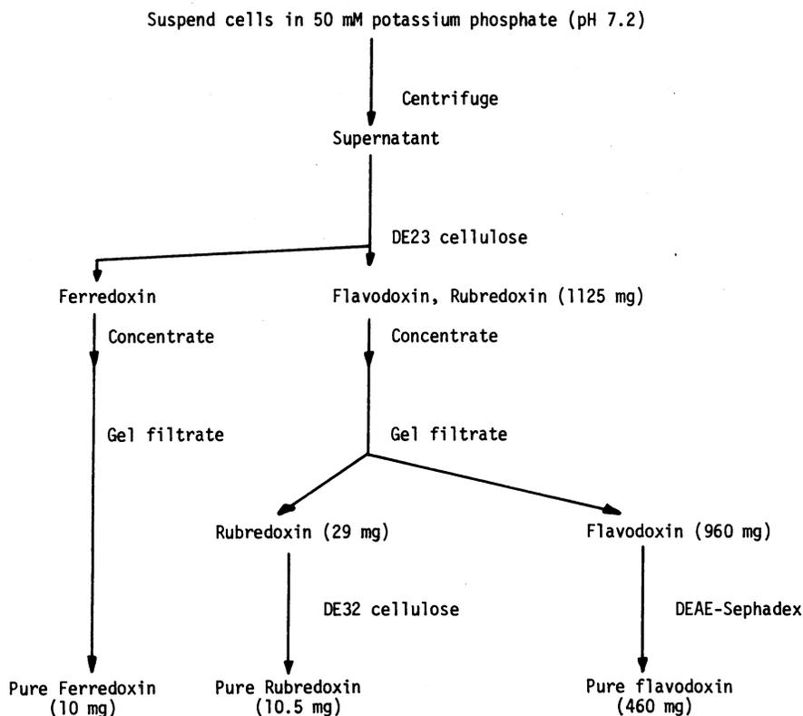
FIG. 1. Purification of rubredoxin, flavodoxin, and ferredoxin from 205 g of *C. formicoaceticum* cells grown in low-iron medium. The final yields of ferredoxin and flavodoxin were dependent upon the concentration of iron in the medium. See the text for details.
