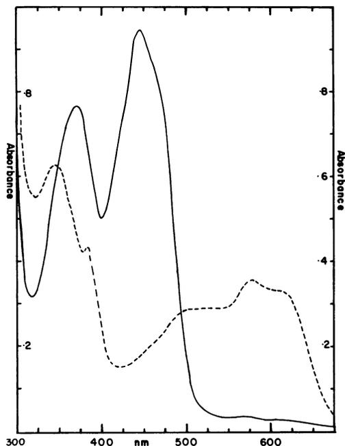
FIG. 3. Light absorption spectrum of *C. formicoaceticum* flavodoxin, 1.80 mg/ml, in 50 mM Tris-hydrochloride, pH 7.6. Oxidized flavodoxin (—) was enzymatically reduced with *C. thermoaceticum* CO dehydrogenase (---) by bubbling with CO for 5 min before addition of enzyme.
