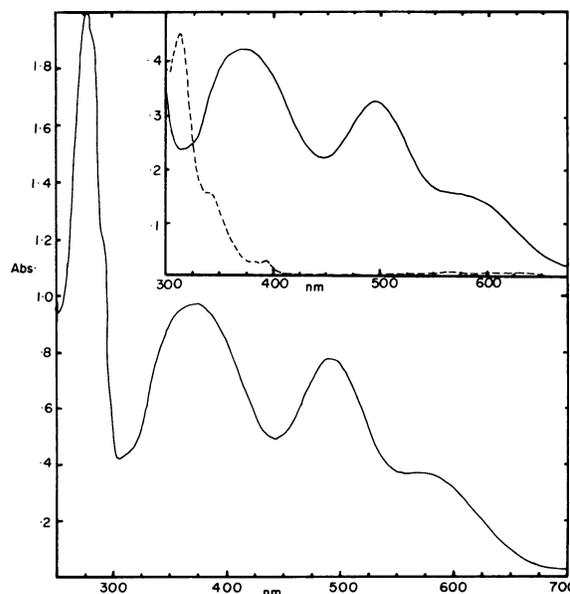
FIG. 2. Light absorption spectrum of *C. formicoaceticum* rubredoxin, 0.64 mg/ml in 50 mM Tris-hydrochloride, pH 7.6. Inset shows rubredoxin, 0.25 mg/ml, oxidized (—) and enzymatically reduced with *C. thermoaceticum* CO dehydrogenase (---) by bubbling with CO for 5 min before addition of enzyme.
