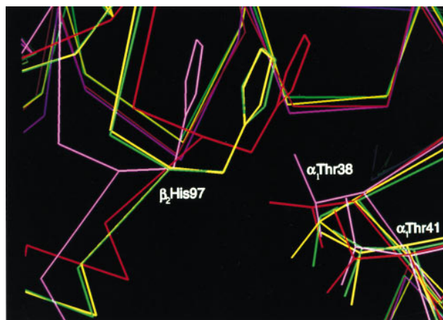
FIG. 4. The switch regions of \alpha_2\beta^{82}CA^{82}\beta (yellow), \alpha_2\beta^{82}ND^{82}\beta (green), R2 hemoglobin (magenta), and R hemoglobin (red) after the superimposition of the \alpha_1\beta_1 interface as described (1), revealing the intermediate characteristic of the cinnamyl and naphthalenyl crosslinked hemoglobins.
