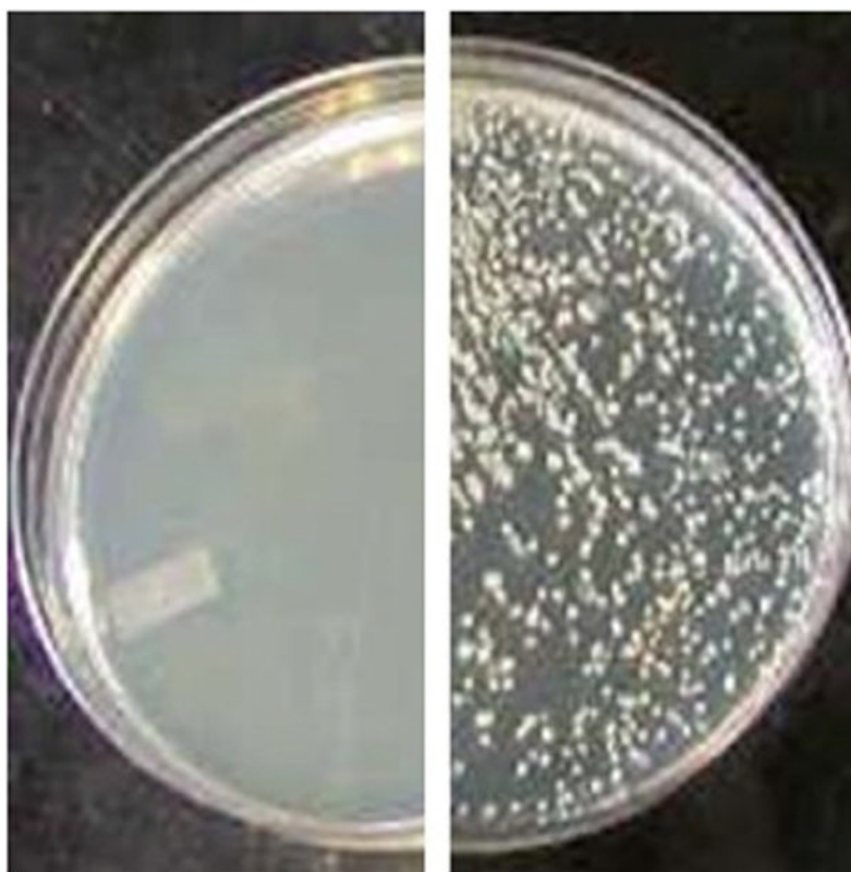
Fig. 17. Photographs of modified medical grade PVC from catheter tubing (blended with AMM), ( Left ), and unmodified PVC, ( Right ), after spraying with aqueous suspensions of S. aureus cells ( 10^5 cells/mL), air drying for 3 min, and incubating under rich growth media at 37 °C for 24 h.
