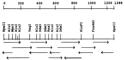
FIG. 5. Sequencing strategy for pSN2 DNA. Both the strands were sequenced. Numbers refer to base pairs. Arrows indicate the direction and extent of sequence determination.
