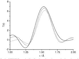
FIG. 9. HEXRD pair-distribution functions of phosphate-based glasses Ag10 (solid line), Ag15 (dashed line), and Ag20 (dotted line) showing the peak due to P—O bonding.
