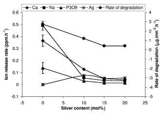
FIG. 6. Relationship between cation and anion release rates and rate of degradation of silver-doped phosphate glasses as a function of silver content.
