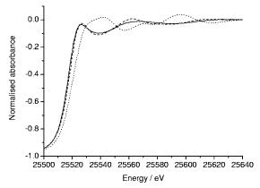
FIG. 10. Ag K-edge XANES spectra: Ag10 glass (solid line),  $Ag_2SO_4$  (dashed line), and AgO (dotted line).
