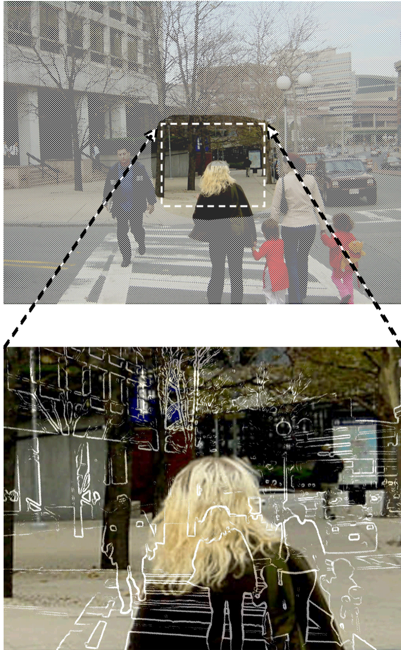
Figure 1. Simulation of a street-crossing scene as it might appear to a patient with tunnel vision using an augmented-vision visual field expander. The faded area in the wide-scene picture (upper panel) represents the peripheral field that patients with tunnel vision typically cannot see when looking straight ahead. The picture in the lower panel provides a magnified representation of the display area and the view seen through the display. The natural (see-through) view is observed in full resolution, while the superimposed minified edge images provide a wide field of view enabling detection of all the pedestrians (not just the lady in the see-through view), which could be potential collisions not visible without the display.
