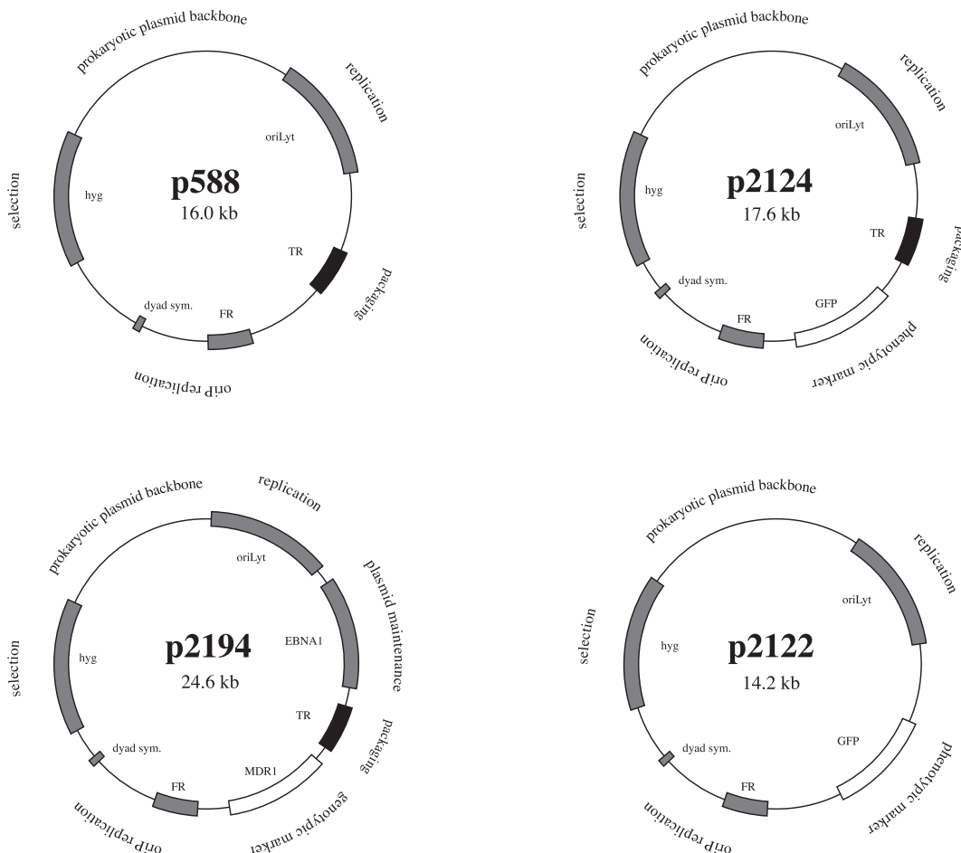
FIG. 3. Schematic representation of the various plasmids used in this study. All plasmids are derived from the p588 plasmid (8) that consists of the two replication origins, oriP and oriLyt, the TR packaging-signal sequences, the EBNA1 gene, and the hygromycin-resistance gene (hyg). The other constructs carry a phenotypic marker (GFP in p2124 and MDR1 in p2194) or lack the TR packaging-signal sequences, as in p2122.
