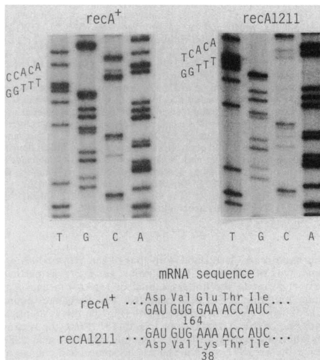
FIG. 1. Comparison of the portions of DNA-sequencing gels for recA1211 (Prt c ) and recA + that show the change in base 164 (codon 38) that occurred in the DNA of recA1211 . The standard Sanger dideoxy method was used.
