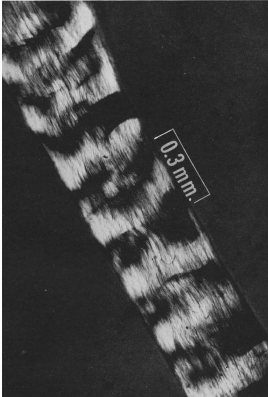
FIGURE 2. A wet unstretched rat tail tendon photographed under polarized light.
