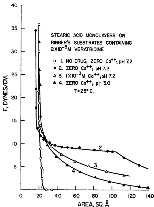
FIGURE 6. The antagonism of the veratridine-stearate interaction by low pH and  $\text{Ca}^{++}$ .
