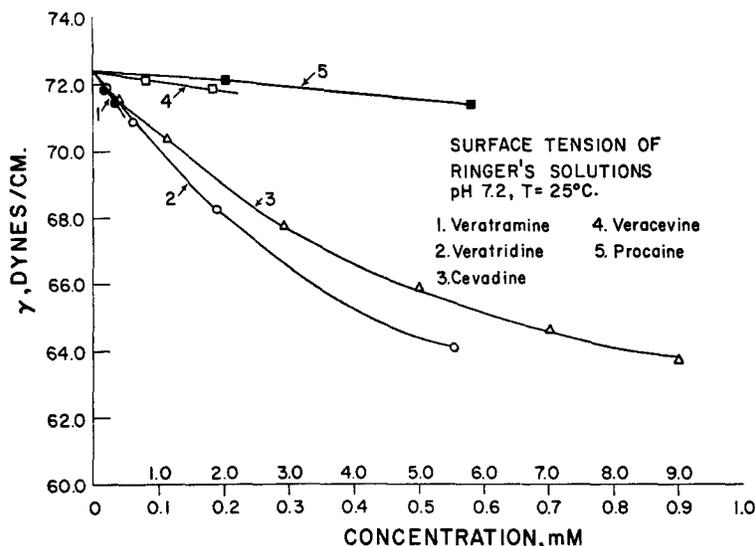
FIGURE 2. Lowering of the surface tension,  $\gamma$ , of Ringer's solutions by the pharmaceutical agents. Curves 1, 2, 3 lower scale, curves 4, 5 upper scale of abscissa.
