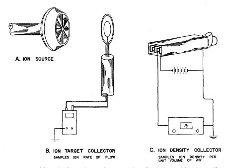
FIGURE 1. Methods of quantitation for gaseous ions. Ions generated by A are collected on surface of target probe B providing a measure of numbers of ions/cm<sup>2</sup>/sec. or are measured as numbers of ions/cc of ambient atmosphere by ion collector C.
