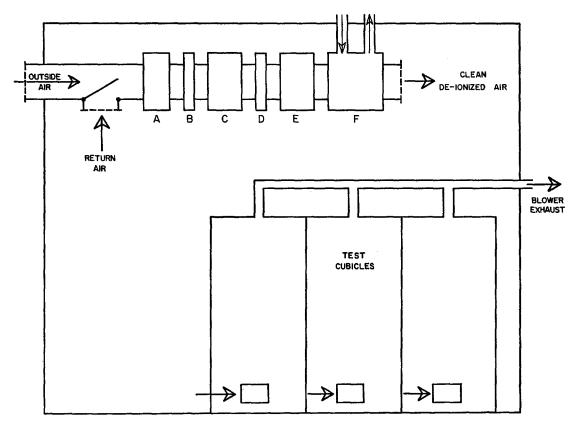
FIGURE 2. Diagram of air purification unit designed to provide clean air for gaseous ion investigations. A, electric duct heater. B, prefilter for C. C, electrostatic precipitator. D, negative ion source to neutralize excess positive ions generated in C. E, activated carbon filter. F, air conditioner.
