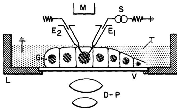
FIGURE 1. Diagram of set-up. *L*, lucite box. *V*, optical glass. *T*, Shen's solution. *G*, isolated gland. A gland contains about 200 cells, a few of which are drawn out of proportion. *E*<sub>1</sub> and *E*<sub>2</sub>, Ling-Gerard microelectrodes driven by micromanipulators. *M*, microscope with darkfield and phase contrast condensers (*D-P*).
