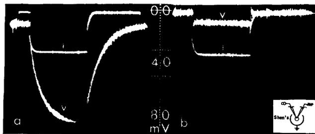
FIGURE 7. Nucleus resistance after destruction of the nuclear membrane. Square pulses of  $1.5 \times 10^{-6}$  A (*i*) are passed into a semiisolated nucleus from a large ground electrode in the Shen's solution in contact with the open cytoplasm (current density =  $39.5 \times 10^{-3}$  A/cm<sup>2</sup>); the resulting voltage drops (*v*) are recorded before (*a*) and after (*b*) drilling a hole into the nuclear membrane. Time calibration 1 msec.
