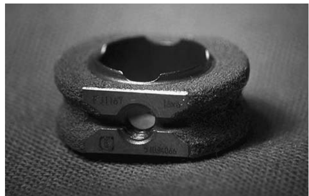
Fig. 1 Cervical intervertebral device evaluated in this study. The Cespace® has a rectangular box design with central opening that can be filled by cancellous bone or bone substitute. The porous coating of both superior and inferior aspects converging in 5° should facilitate bony ingrowth
