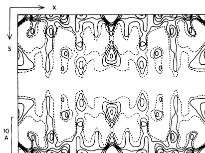
FIG. 3.— (hkk) Patterson projection for type B crystals. The letter s designates a vector lying in the b, c plane, and at an angle of approximately 41^\circ to c . Contours are at equal arbitrary intervals. The dashed contour is the “zero” contour; “negative” contours are omitted.
