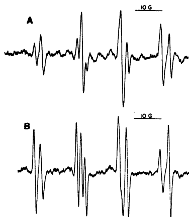
FIG. 3. EPR spectrum obtained by incubating the spin trap DMPO with M. formicicum in the presence of formate (10 mM). Scans were initiated 30 s (A) and 25 min (B) after the reaction had begun. Microwave power was 20 mW, and the modulation frequency was 100 kHz with an amplitude of 0.63 G. Sweep time was 12.5 G/min, and the receiver gain was 12,500 with a response time of 1 s.
