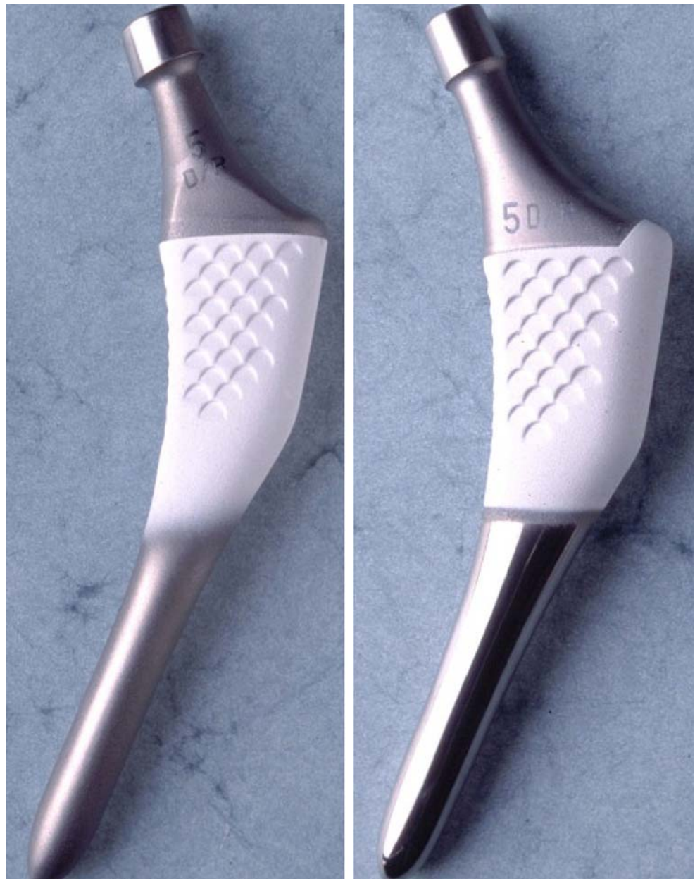
Fig. 1 Stryker ABG-I ( left ) in comparison to the Stryker ABG-II ( right ) implant made of a low modulus titanium alloy and having a shorter small-diameter polished stem, increased proximal HA coating and neck lateralization ( 130^\circ vs. 135^\circ )
