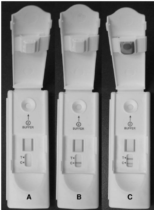
FIG. 2. Assay procedure and results. (A) Device run with buffer only. (B) Device run with an HSV-2-negative serum. (C) Device run with HSV-2-positive whole blood.
