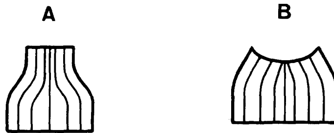
FIGURE A1. Schematic indication of the fiber orientation in two kinds of fiber-optic taper. (A) Standard magnifier/condenser: fibers perpendicular to two flat surfaces. (B) Fiber-optic taper used for these studies. Note how fibers are approximately normal to curved surface.
