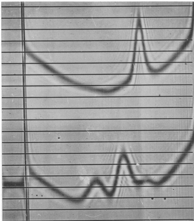
FIG. 1.—Ultracentrifuge patterns of \gamma component (upper curve) and, for comparison, a mixture of \alpha , \beta , and \gamma components (lower curve).
