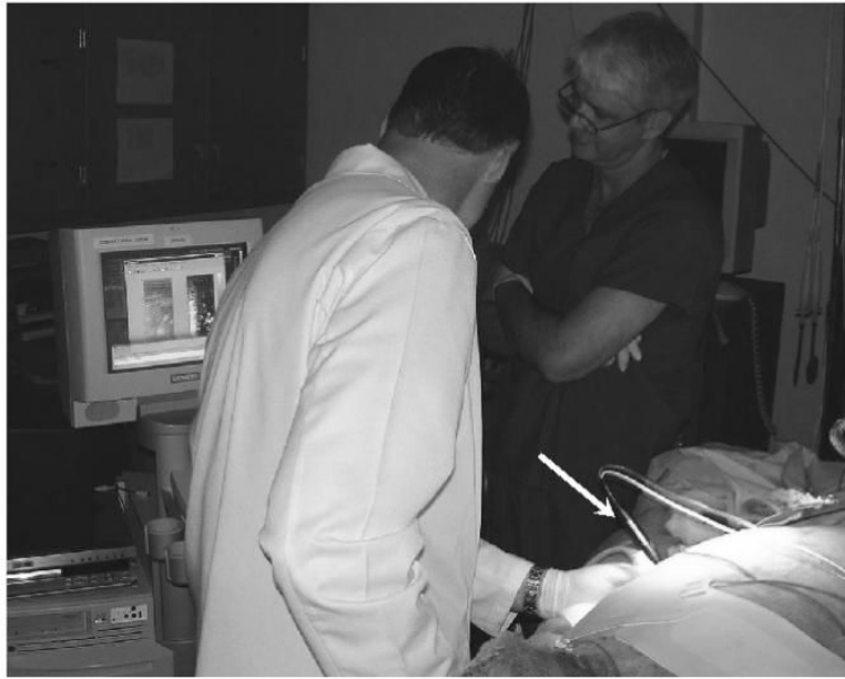
Figure 6. Example of real-time implementation of ARFI monitoring of RF ablation in vivo . B-mode and ARFI images are acquired and displayed in real time on the monitor of the ultrasound scanner. White arrow points to the ablation electrode after its insertion into the animal's liver.
