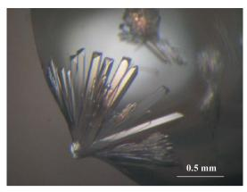
Figure 2 Photograph of AD2<sub>PF-ChiA</sub> crystals grown by the hanging-drop vapour-diffusion method. A crystal of  $0.1 \times 0.1 \times 0.5$  mm in size was used for X-ray analyses.
