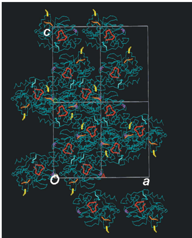
Figure 4 Crystal-packing diagram of the ac plane in the NaCl/Tris crystal. Tris (magenta) and the structurally unique regions A (yellow), B (orange), C (red) and D (blue) form a diagonal line in the ac plane.
