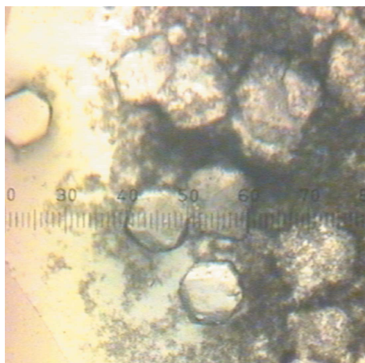
Figure 3 Crystals of apo-GpdQ in 1.9 M sodium malonate pH 7.0. The scale is 0.025 mm per gradation.
