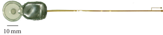
FIGURE 4: A photograph of retinal electrical stimulator which consists of receiver coil, hermetically sealed metal package, and polyimide-based active and reference electrodes.
