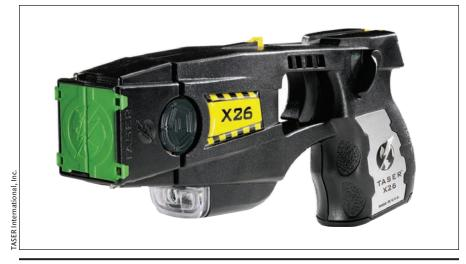
The TASER X26 stores time, date, duration, temperature and energy cell status of over 1500 firings. Powered by lithium energy cells with a 10-year shelf life, the X26 is the taser of choice for most police departments and retails for US\$799. TASER International, Inc., says it has sold the devices to 175 Canadian law enforcement agencies.
