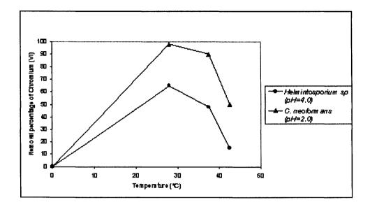
Fig. 3: The effect of the incubation temperature on the biosorption on chromium (VI). 0.2 mg/L, 80mg biomass, 24 h of incubation with constant agitation.
