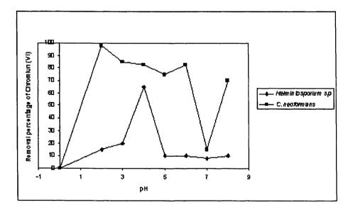
**Fig. 2:** The effect of pH on the biosorption of Chromium (VI). 0.2mg/L/100mL/80mg biomass, 28°C, 24 h of incubation with constant agitation.
