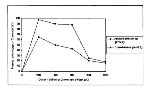
Fig. 4: The effect of the concentration of chromium (VI) in solution on the biosorption 80 mg biomass/ 100mL, 28°C, 24 h of incubation with constant agitation.
