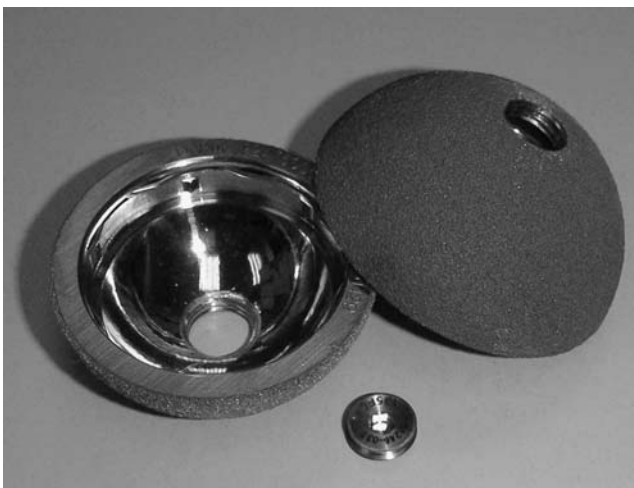
Fig. 1 The Duraloc 100 Polished HA acetabular component has hydroxyapatite plasma sprayed onto the porous coating. There is no screw hole and no stabilising spike or peg. The apex hole can be plugged to occlude access of polyethylene wear debris into the acetabular fixation interface
