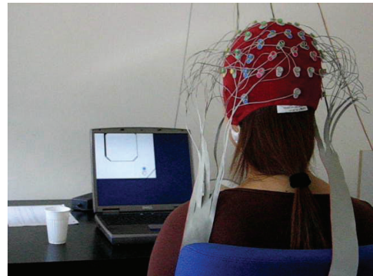
FIGURE 5: A subject controlling an intelligent wheelchair in a simulated environment. Visible is the EEG sensor cap with the cables that are connected to the BCI system and the computer that runs the shared control system.
