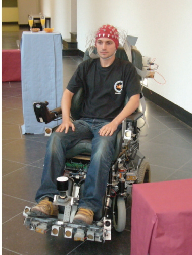
FIGURE 1: A subject controlling our robotic platform Sharioto in a natural indoor environment through noninvasive EEG. Visible are the sensors of the platform: a laser range scanner in front and sonar sensors all around.
