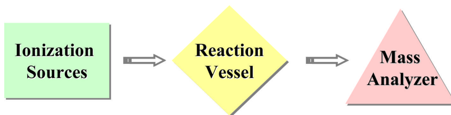
Scheme 1. Instrument components for ion/ion reaction studies.
