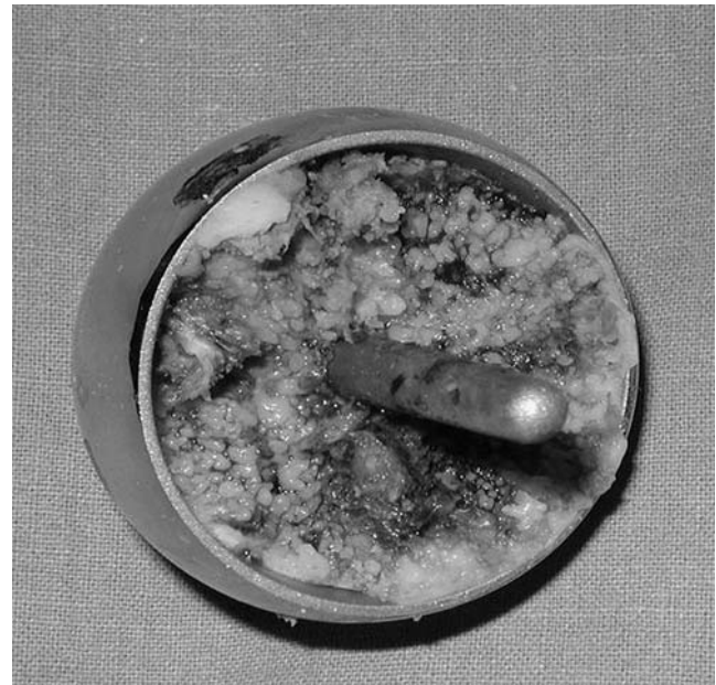
Fig. 5 Retrieved specimen. Massive cement penetration into the proximal femoral epiphysis
