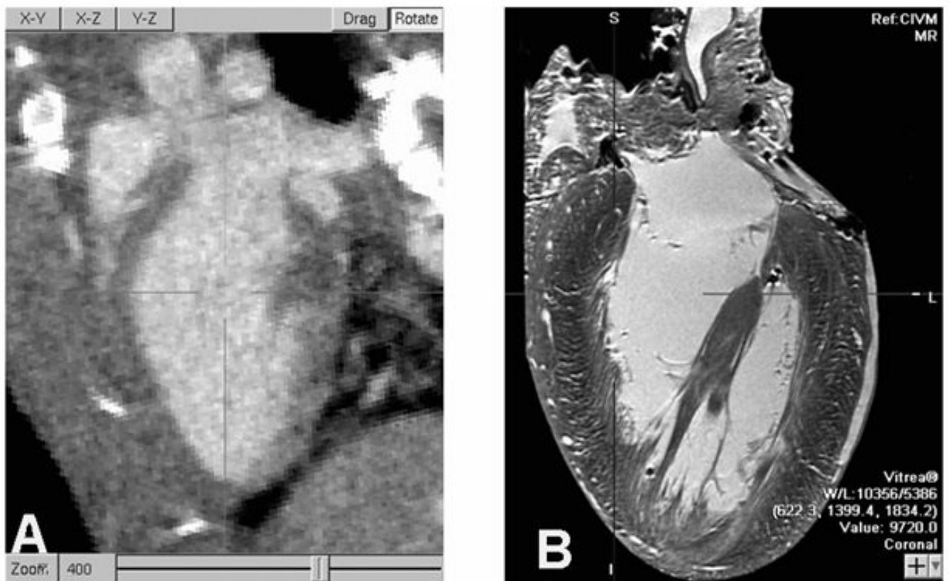
Fig. 2. An oblique slice through reconstructed 100 micron/voxel micro-CT from a live mouse, on the left, shows the LV blood highlighted by contrast agent and motion blur suppressed due to 10 ms x-ray pulse width. MRM imaging of a fixed heart at 20 micron resolution, at right, reveals substantial anatomical detail that cannot be resolved in live mouse imaging. High precision measurements of LV blood volumes have to account for these unresolved features. (Note: The micro-CT is digitally zoomed to 400%.)
