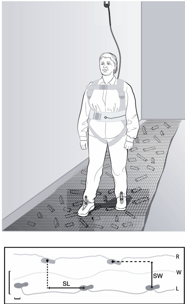
Figure 1. Schematic diagram of the irregular surface, marker placement and definitions of step width and length
