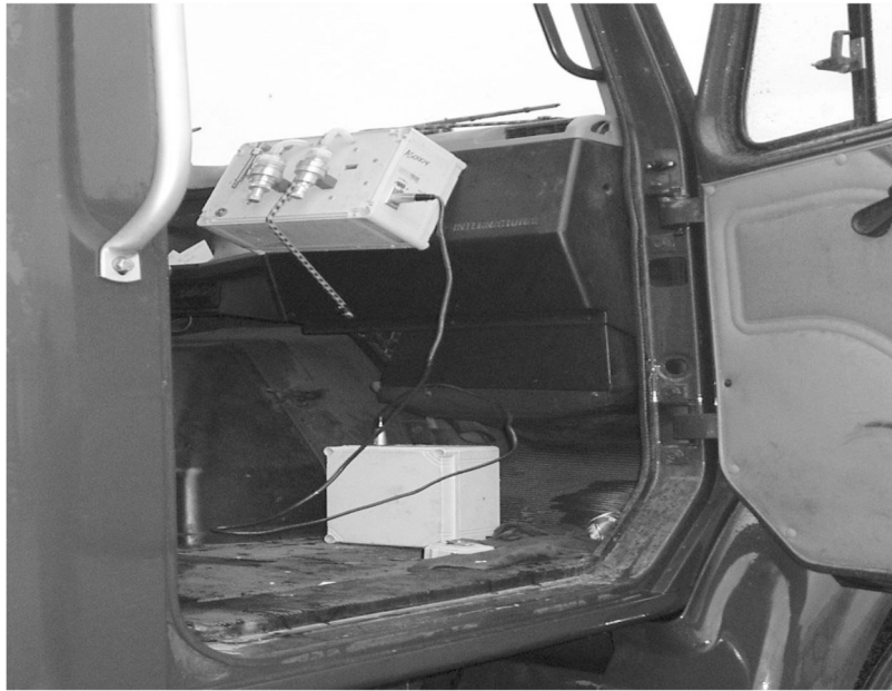
FIGURE 1. Sampler box setup in truck cab
